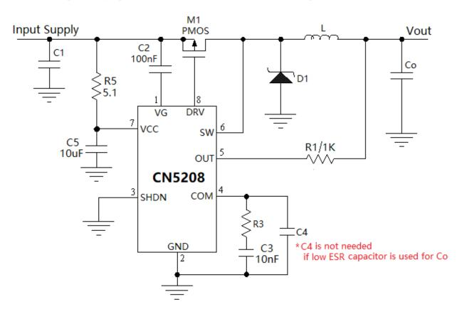
Figure 3 Protect CN5208 from Input Voltage Spike
